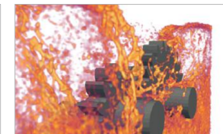
Instantaneous splashing of oil in a gearbox
