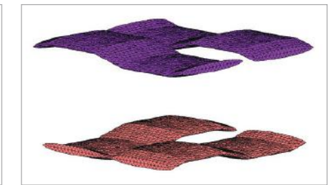
Laminate from stack of homogenous plain weave unit cells of multiple orientations
