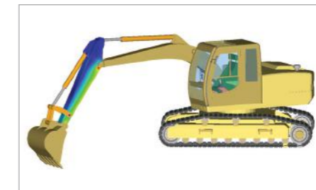
Excavator flexbody simulation
