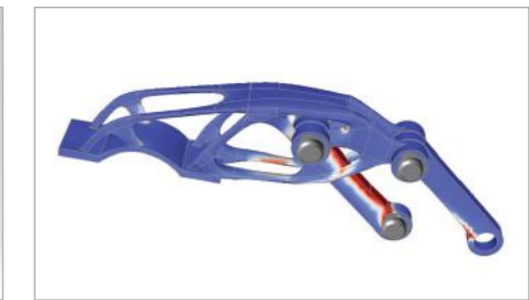
Analysis of an optimized robot gripper arm
